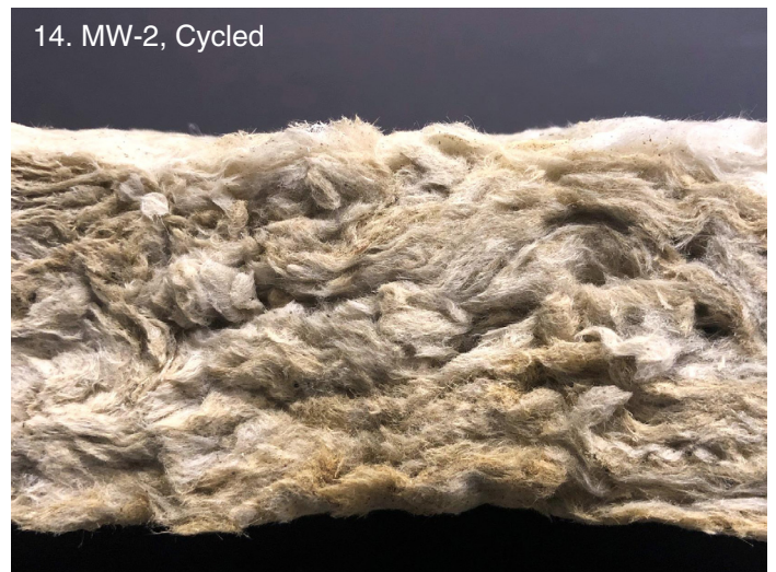
Figs 11-14. Changes in slab macrostructure in response to rewetting. Cycled specimens exhibit separation of fiber layers and notable voids. Cycled slabs also show evidence of reduced tensile and compressive strength.
