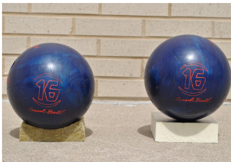
The above image shows the lack of compressive strength of mineral wool compared to Polyiso. Standard 16lb bowling balls were used with 6"x6" samples.
